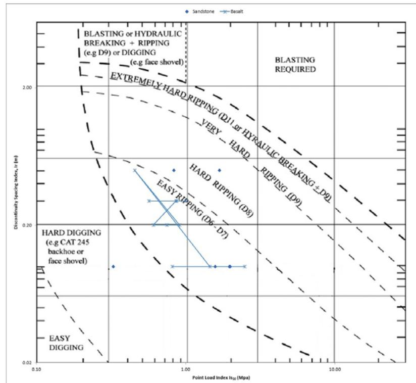
Figure 5: Rock Strength vs Excavatability (Tsiambaos, 2009)
