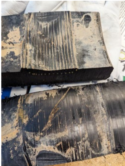
EF failure with suspected Bentonite contamination and severe gouge
