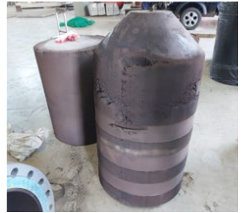
Figure 2: Foam pigs used for displacing liquid
