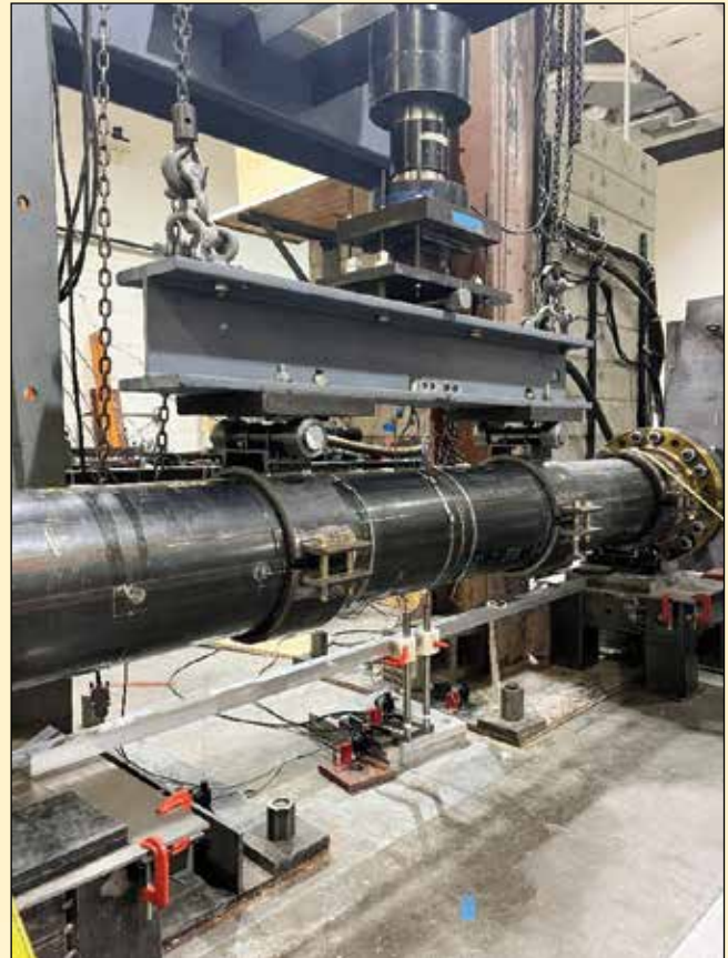
12-inch steel pipe lined with ALTRA10™ undergoing lateral load testing
