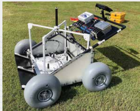
APEX surface pushcart detects, locates, and classifies underground pipes
