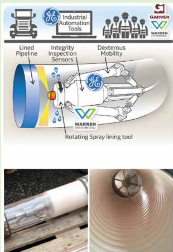
The PLUTO system tightly integrates industry leading capabilities in robotic mobility, asset inspection and pipe lining material application
