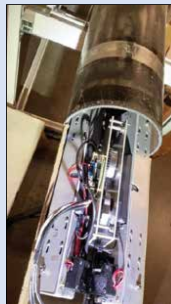
Current version of the fiber optic deployment tool (FODT) entering an 8-inch pipe during a 50-foot demonstration of fiber optic sensor installation along pipe interior
