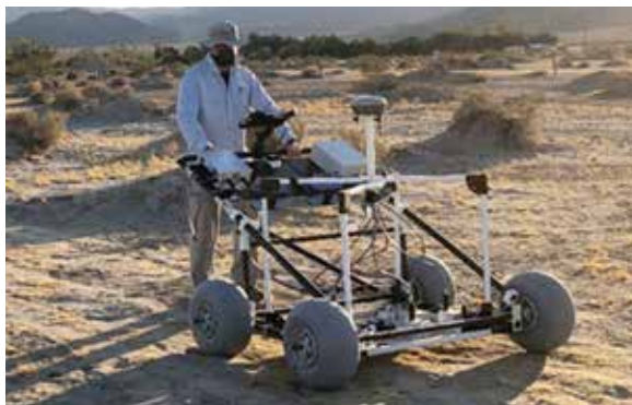
Figure 1. APEX Advanced 3D Sensor is a Person-Portable System Developed to Detect and Characterize Subsurface Objects
