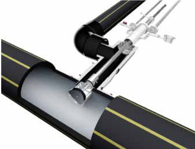
Figure 4 – Cutter Tapping PE Main Under Pressure
