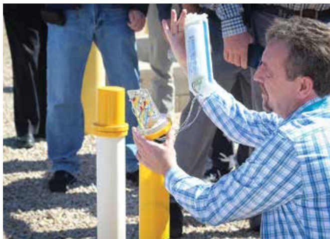
Remote corrosion monitoring device fits inside standard test point markers
