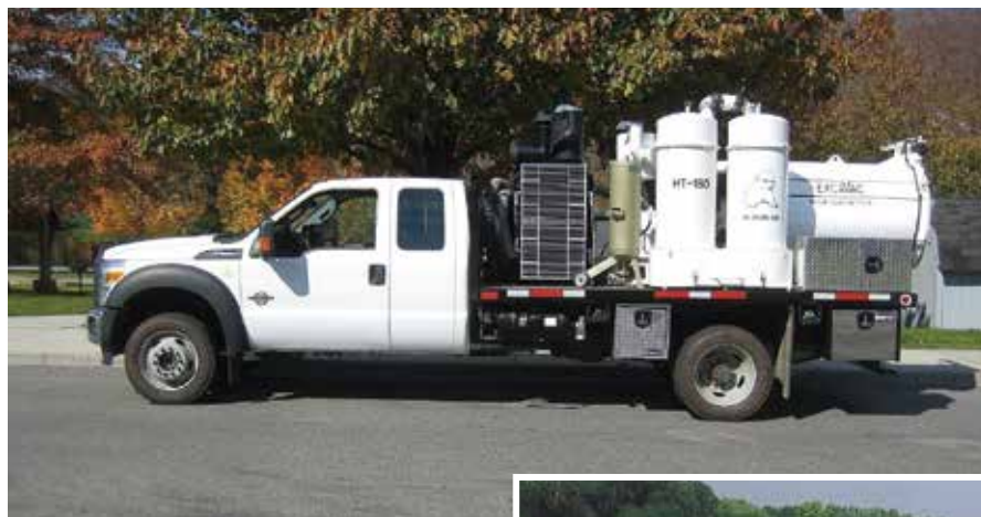
Air/Vac system on 4x4 extended cab chassis
