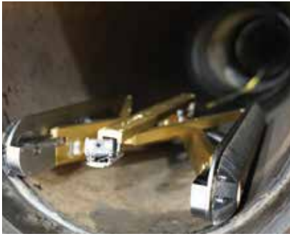
M1 Live Gas Main Inspection Crawler System
