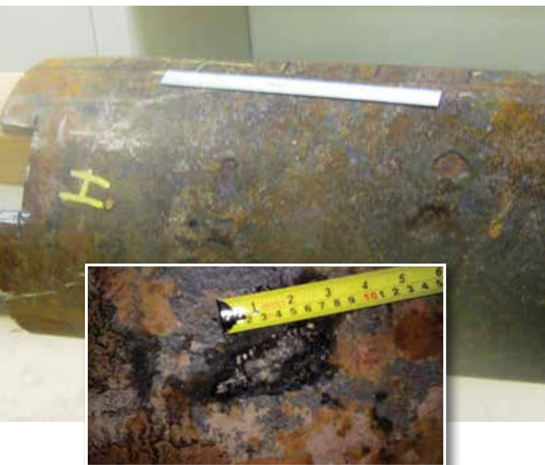
Figure 1: Cast iron gas pipe graphitic corrosion and pitting [Source: Final Report, GTI Project Number 21874; p9.]
