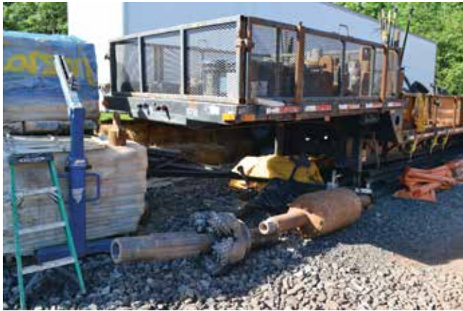
24-inch Reamer and Swab. Approx. 300,000 gallons of water were used during the pilot and reaming operations
