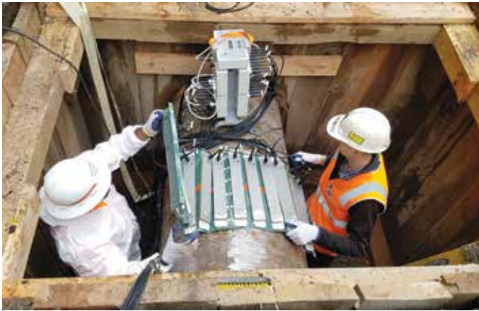
Figure 5. Sensor blanket for BEM external Flexible Array Scanning Tool (FAST) wraps around the pipe
