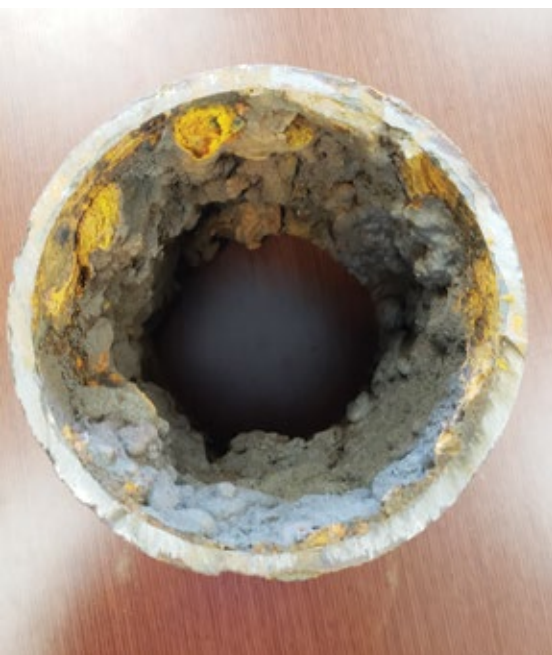
Significant tuberculation in the host pipe
