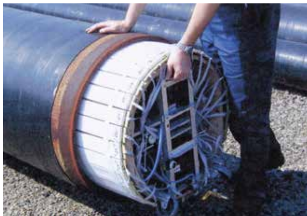
Internal pig probe with multiple sensors
