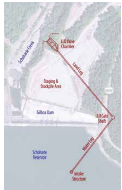
Figure 2: Low Level outlet tunnel alignment
