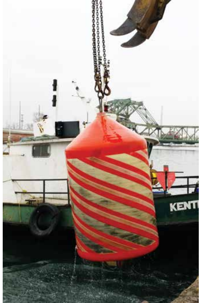
Figure 6.60-inch brush pig after being towed to shore
