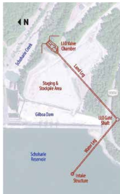
Figure 2: Low Level outlet tunnel alignment
