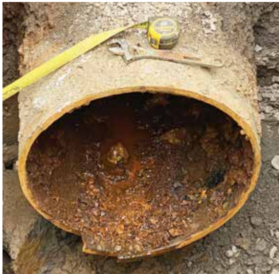
Pre Rehab Tuberculated Pipe
