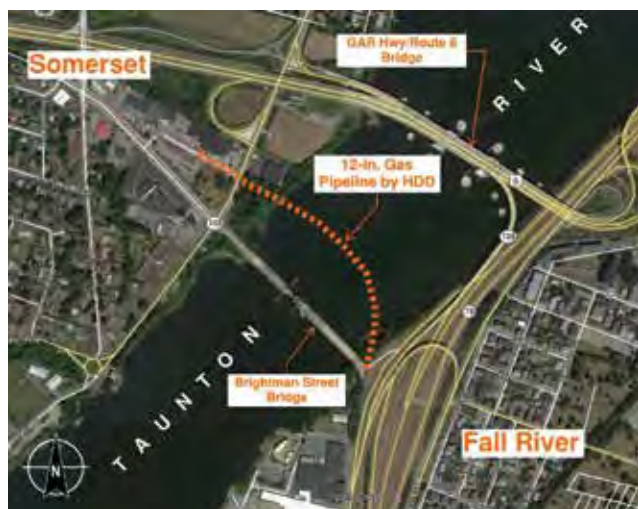
Figure 1 – Plan of 12-inch gas pipeline installed in 2016/2017 by HDD below the Taunton River. Base image from Google Earth Pro, dated 26 Feb 2018.
