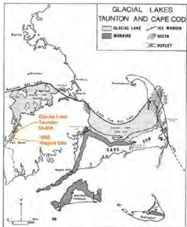
Figure 2 - Glacial Lake Taunton impounded against ice front or moraine formed by Buzzards Bay ice lobe. Outlet channel and HDD project shown (Modified from Larson, 1982, Fig. 3).
