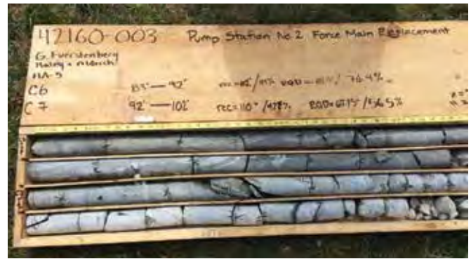
Figure 6: Sample rock core showing Precambrian Gneissic bedrock
