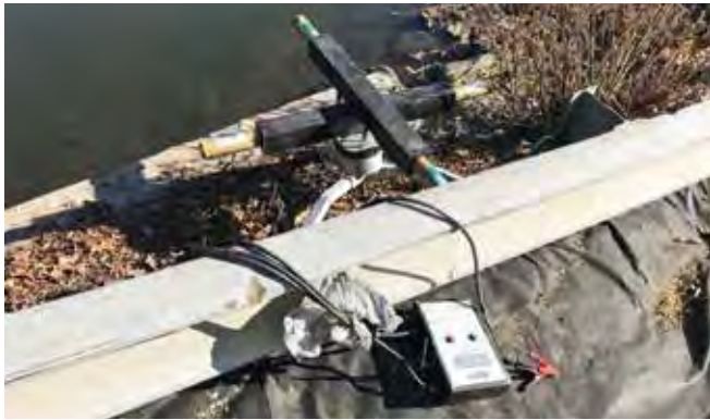
Figure 9: The Magnetic Beacon system
