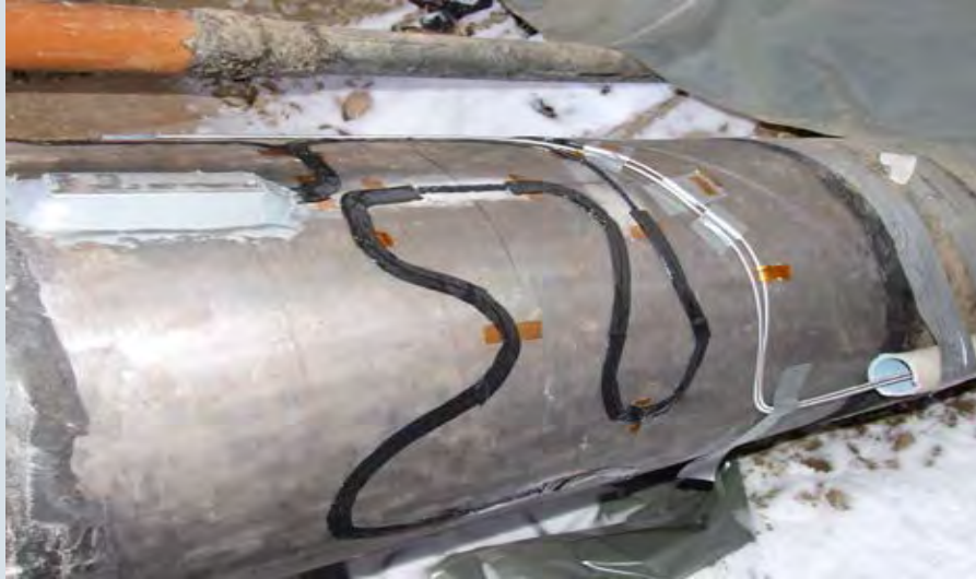
HBM- Fiber Optic Strain Sensors Monitor Pipeline Integrity, www.hbm.com/en/4577/fiber-optic-strain-sensors-monitor-pipeline-integrity/
