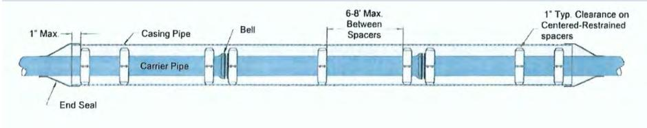
**A. General Carrier**: One spacer shall be placed not more than one foot from each end of the casing and pipe joint. Subsequent spacers shall be a maximum of 7' intervals within the casing.
